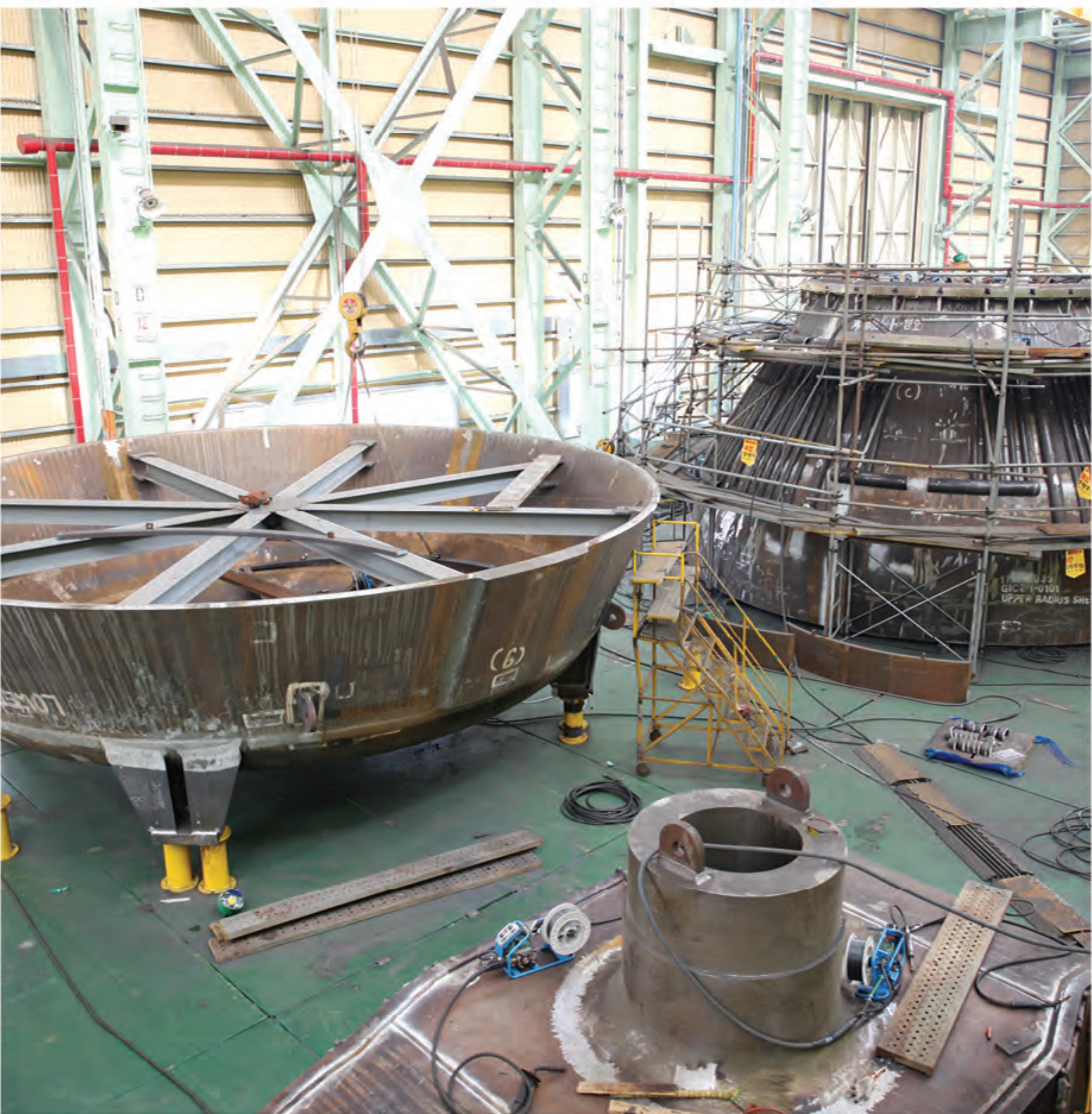
Manufacture of a converter at the New port Manufacturing Plant
