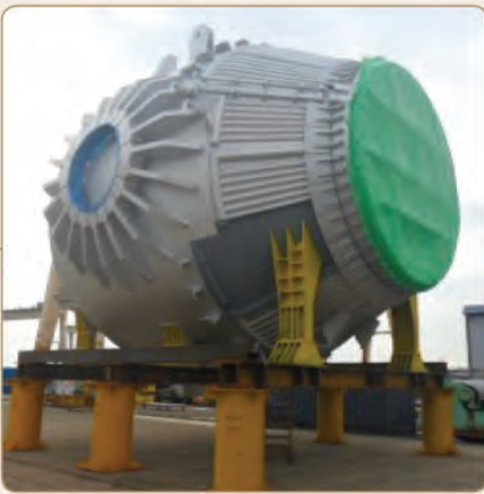
Gwangyang) 2 Steelmaking 1 Converter Trunnion Ring & Converter Vessel
